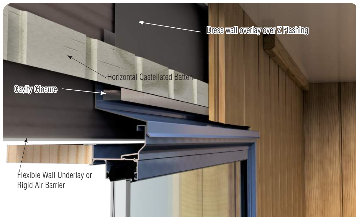
Typical Window and door Detail
